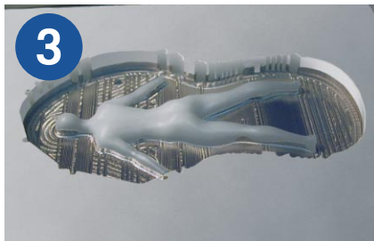
Right: After hardening, workpiece is turned over and machined on reverse side
