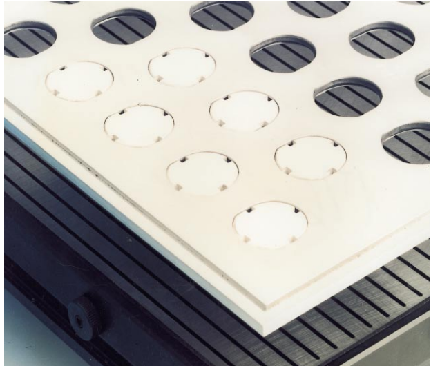
Slot vacuum chuck with special adapter plate
