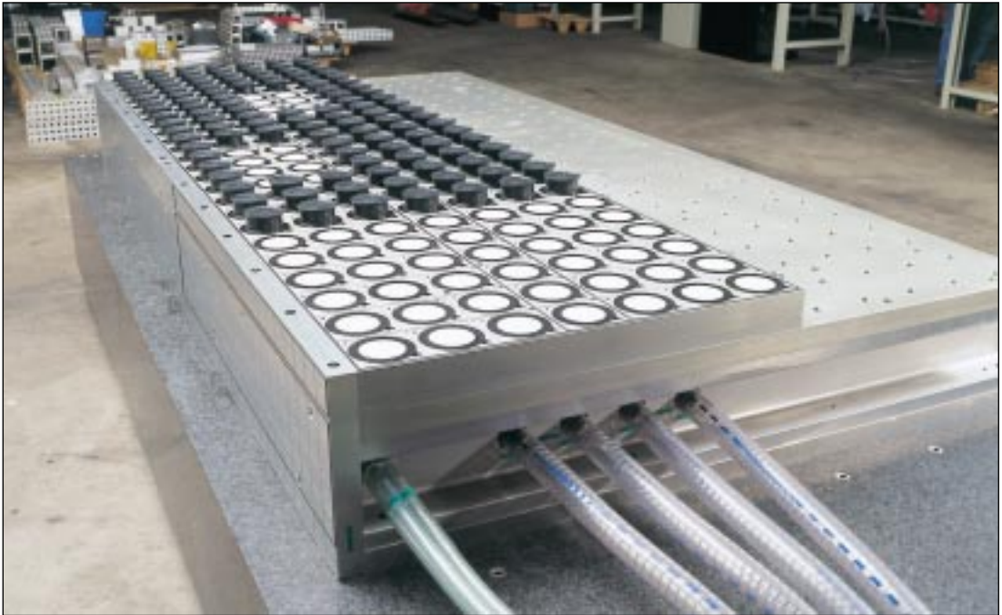
FLIP-POD™ clamping system in working position prepared for a large aluminium workpiece with cutouts
